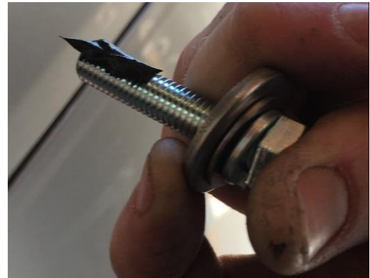
Figure 16: Silicone Sealant Applied to the M8 Mounting Hardware
